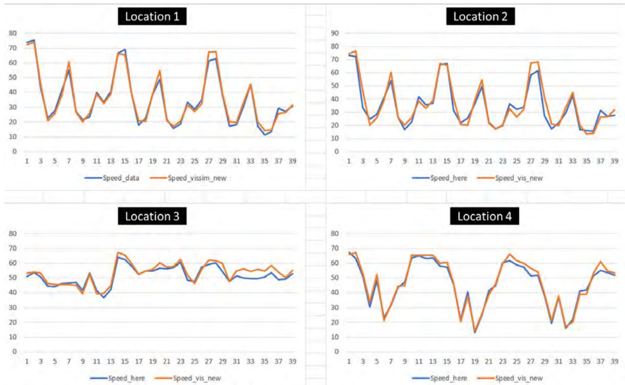
Figure 4-5 Calibration Results for VISSIM Roadway Geometry
